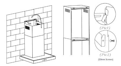
Fit the chimney fixing plate to the wall and attach the chimney section to the plate
