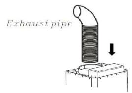
Now secure the chimney section(s) to the cooker hood body as shown below in Pic.1 ensuring that you secure with the 2 screws as shown in Pic.2.
