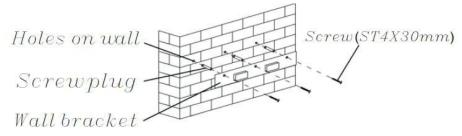
Hang the cooker hood onto the wall bracket and secure
