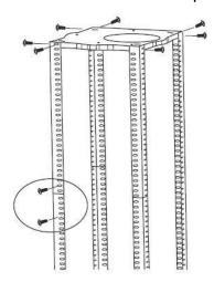
If you are going to use the hood in extraction mode, you should connect the flexible house to the vent outlet at this point in the installation. Fit the upper chimney section to the ceiling plate and secure with the 4 x screws.
