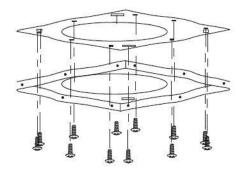
Fit the angle bars to the ceiling plate using the 8 x M5 screws and then extend the bars to the required length and secure using the 16 x M5 screws. N.B. the bars must have an overlap of at least 100mm.
