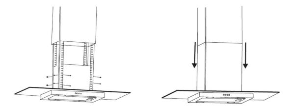
The cooker hood should ideally be installed between 65-75cm above the work surface/cooker hob. DO NOT INSTALL BELOW 65cm.
