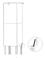
Lift the lower chimney section onto the angle bars
