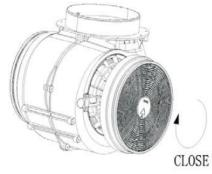
Make sure the filter is 'locked' into position and note that suction power is lowered when using carbon filters.
