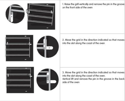
1. Raise the grill vertically and remove the pin in the groove on the front side of the oven
