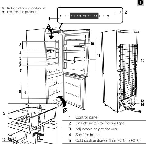
The transparent cold section drawer 5 moves on roller bearings 16. The drawer can be removed by pulling it out, and lifting it off the rails.
