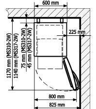
If the appliance is placed in a corner, a gap must be left between the appliance body and the wall so that the freezer compartment door can be opened enough to pull out the frozen product drawer (see picture).
