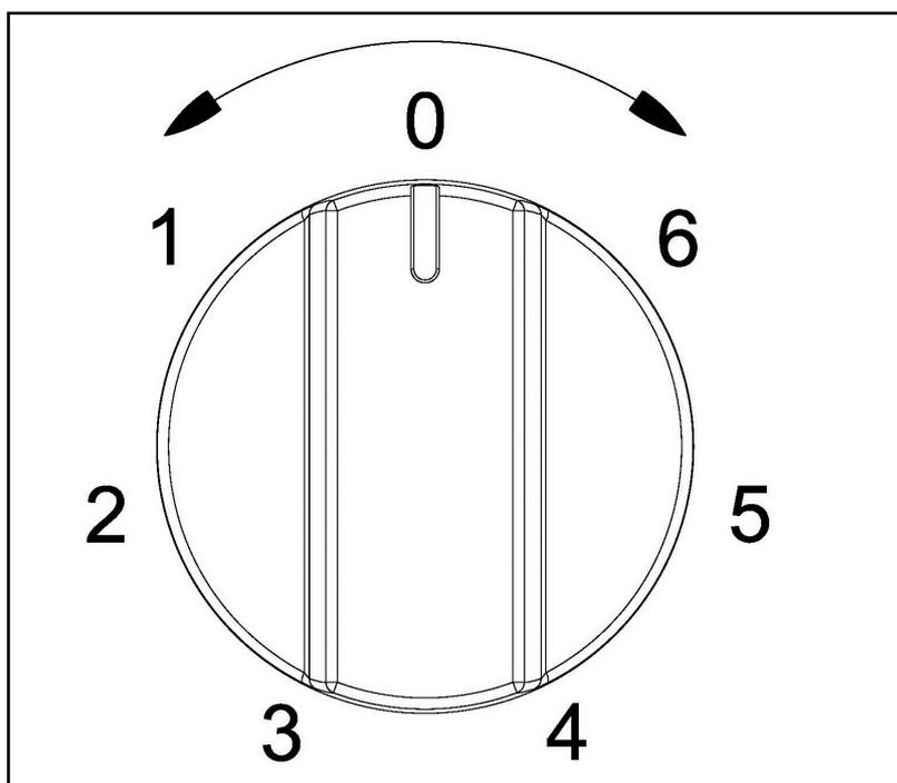
To operate the required solid plate heat zone, simply turn the relevant control knob to the required heat setting, i.e. 1 is low and 6 is high.
