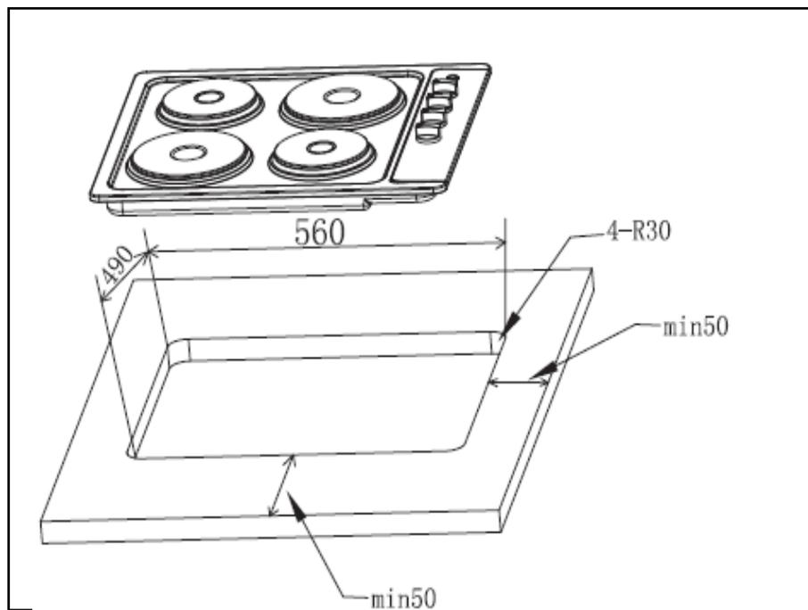
Cut out the opening in the work top for the hob (see diagrams/sizes above).
