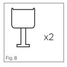
Ensure that the lips of the spacers are level with the lip of the cabinet base.
