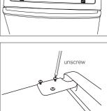
3. Remove the pin with a screwdriver and flip the hinge bracket. Then refit the pin to hinge bracket.
