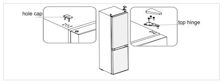
3. Remove the refrigerating door, the middle hinge and the hole caps.
