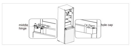
10. Put the refrigerating door on the middle hinge, assemble the top hinge on another side, fix the hinge cover on the top hinge and fix hole cap, as below pictures shows.
