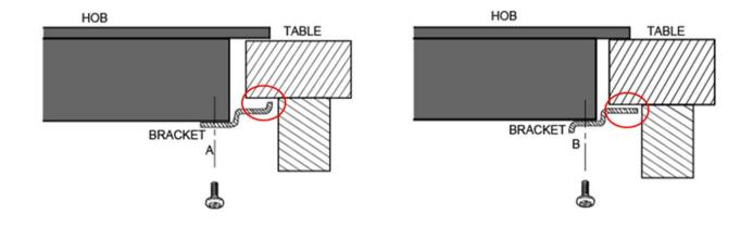
Under any circumstances, the brackets cannot touch with the inner surfaces of the worktop after installation (see picture).
