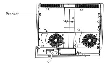
After installation adjust the bracket position to suit for different table top thickness.
